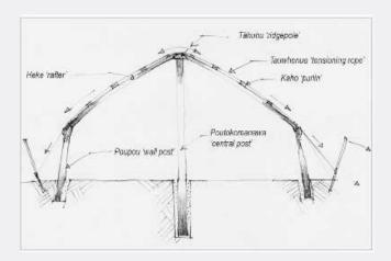
Figure 3: Schematic cross-section of the compressed arched frame of the whare (Treadwell, 2014, p. 96, image used with permission)
